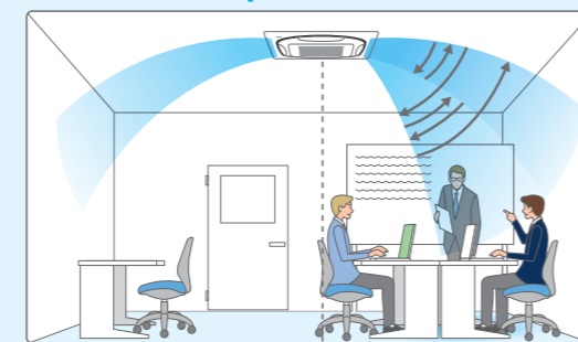
Optimal air direction by "Auto" Swing (narrow)
