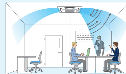
Optimal air direction by "Auto" Swing (narrow)
