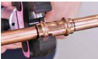
1. Align jaws squarely on the fitting
