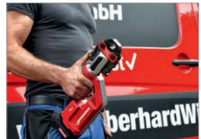
Secondary effect of the two cylinder-structure: The machine can be used with one hand.
