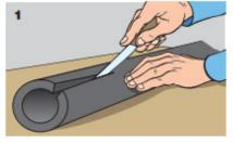
Use only the sharpest knife for cutting - this makes the subsequent glueing far easier.
