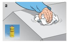
Use thinner to thoroughly clean the surface to be insulated. Insulation is not recommended where there is incrustation or other flaws which could prevent the sheeting from sticking perfectly.
