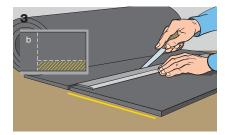
Cut the corresponding portion out of the roll. There is an obvious saving in material by cutting the sheeting along its height (a) rather than along the length of the 1000 mm sheeting (b).
